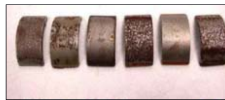
Corrosion appeared on coupons after wet surface tests with 3% KCl, water containing 2 gal/thousand CI-9, and 1% by volume of different corrosion inhibitors. From left to right: Test 21, water-dipped coupon; Test 22 with CI-9; Test 23 with CI-4; Test 24 with CI-6; Test 25 with CI-8; and Test 26 with CI-7 (Fig. 5).
