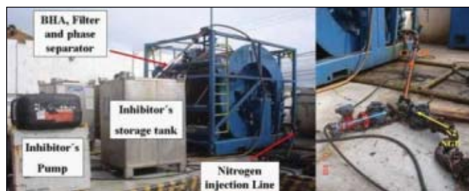
Yard test: While pumping generated nitrogen through the CT string, we dosed with corrosion inhibitor to create an internal film that would protect the pipe from corrosion (Fig. 6).
