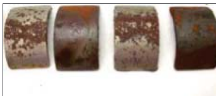
Corrosion appeared on coupons after tests in 3% KCl. From left to right: Test 16, CI-7 dipped coupon, wet surface; Test 17, CI-7 coupon immersed in fluid; Test 19, CI-8 dipped coupon, wet surface; Test 20, CI-8 coupon immersed in fluid (Fig. 4).
