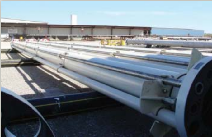
"VetcoGray's HMF risers waiting to be prepared for buoyancy for an operation in the Gulf of Mexico."
