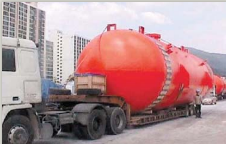
Pressure Vessel for LPG Ship (42t X O.D. 4,000 X L 32,800 : 130ton/set)
