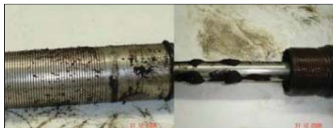
As shown in Fig. 6, the BHA includes a filter and phase separator. The filter has two components: a slotted pipe screen, shown above at left, and smaller diameter magnet, shown above at right. After testing for 3 days at a low N_2 rate, the filter showed a small amount of rust (Fig. 7).
