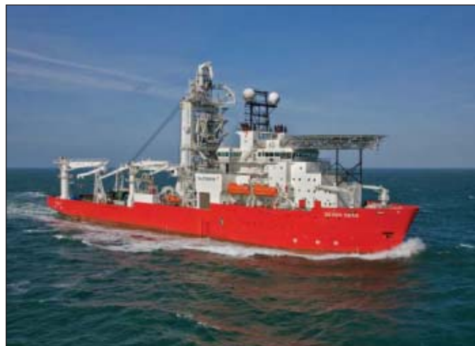
Subsea 7's Seven Seas flex/J-lay vessel. Photo courtesy of Subsea 7.
