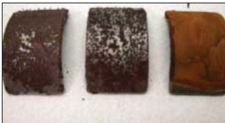
Corrosion appeared on test coupons: corrosion inhibitor (CI)-4 dipped coupon (Test 9, wet surface), CI-6 dipped (Test 14, wet surface), and CI-6 incubated in fluid (Test 15, in fluid); all in 3% KCl brine (Fig. 3).
