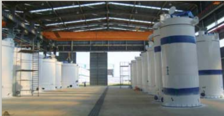
Mud Active Tank for Transocean Project (16t X O.D. 4,600 X H 7,000 : 16ton/set)
