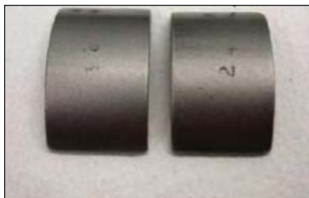
The coupons for tests 11 and 12 appear clean after removal from incubation cells and before sand blasting (Fig. 2).
