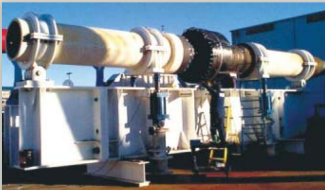
"The Super Heavy Duty connector being tested to 7 million pounds bending capacity at VetcoGray's Houston facility."
